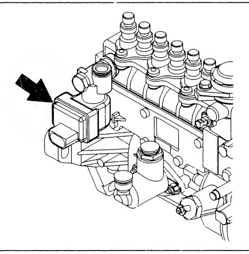
The function of the solenoid valve can only be tested in the vehicle.
